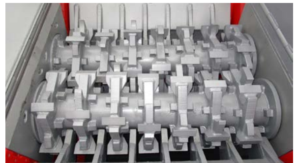
shredding shafts: 1,497 mm
